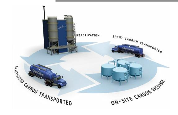
Carbon reactivation is a thermal treatment process in which adsorbed chemical constituents are removed from spent activated carbon and thermally destroyed. Carbon is then reusable and can be returned to service.
